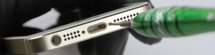
**1** Use **metal pry tool** to remove screen.
