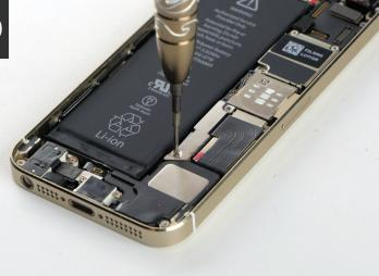
1 Prepare new assembly and plug all (3) flex connectors onto the board as shown in **images 1a-1c**.
