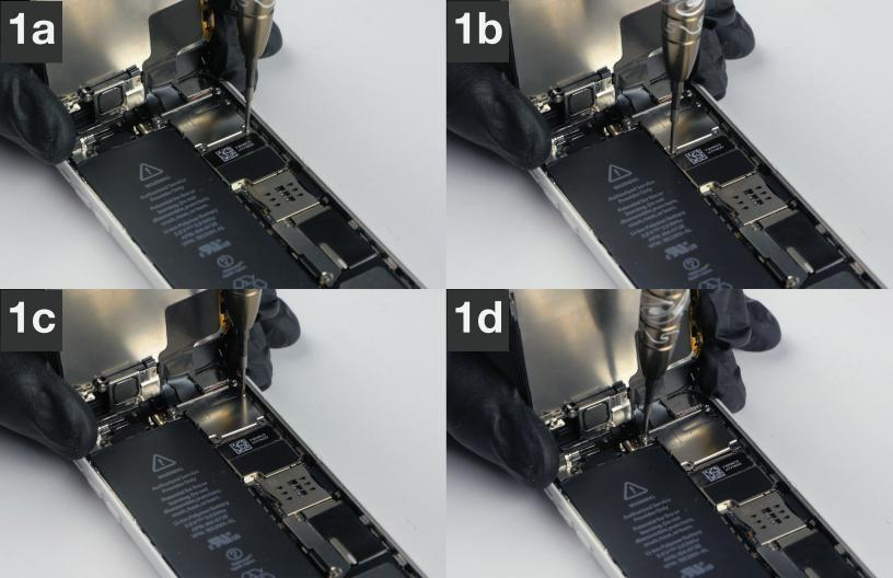
1 Carefully remove the flex shield with **tweezers** as shown in **images 1a-1b**.
