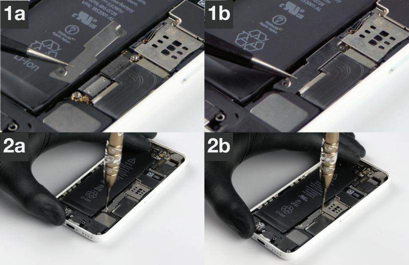
1 Prepare new assembly and plug all (3) flex connectors onto the board as shown in **images 1a-1c**.
